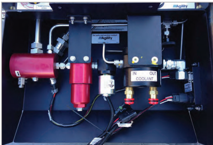
Maintenance-Friendly Mounting Locations for CNG Serviceable System Components
