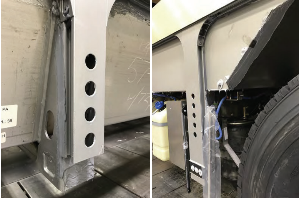
Left: Protected & sealed body/chassis connection. Right: Sealed wheel well and stress panel arch.
