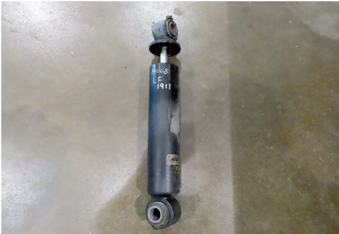
FRONT SHOCK LEAKING (11,491 TEST MILES)
