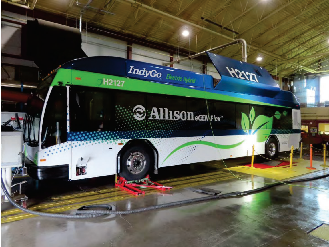
BUS TESTED ON CHASSIS DYNAMOMETER FOR PERFORMANCE, FUEL/ENERGY ECONOMY AND EMISSIONS
