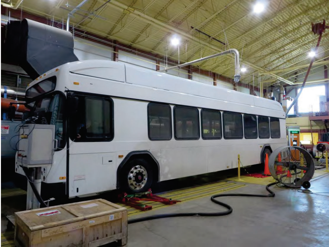
BUS TESTED ON CHASSIS DYNAMOMETER FOR PERFORMANCE AND FUEL ECONOMY
