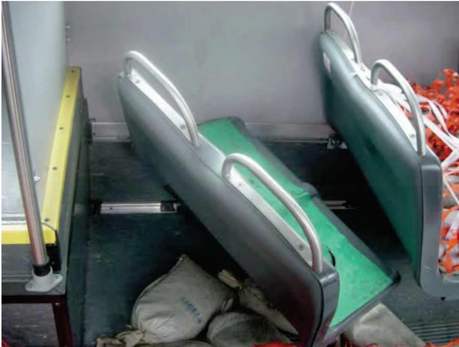
BROKEN SEAT FRAME (5,500 TEST MILES)
