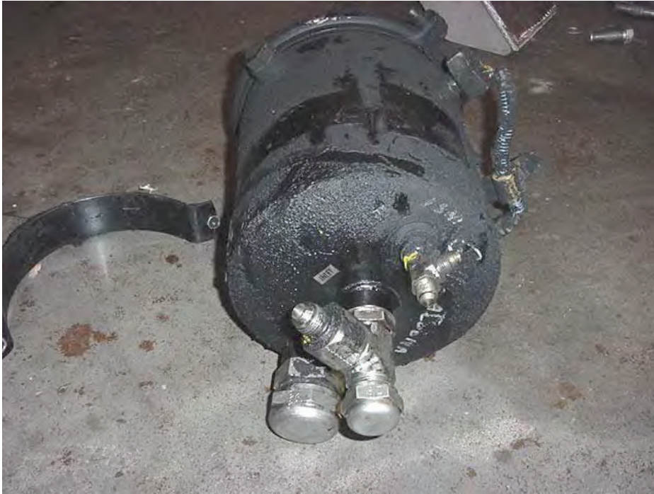
CRACKED HYDRAULIC RESERVOIR (12,487 TEST MILES)
