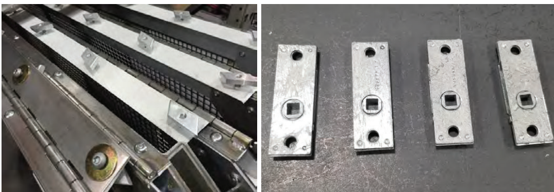
Left: Isolating tape applied over primed hinged panels. Right: Stainless steel square key locks with pre-applied protective coating.
