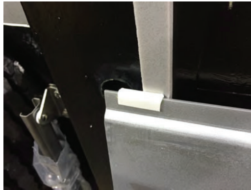
Tape applied to top edge of coated skirt panel
