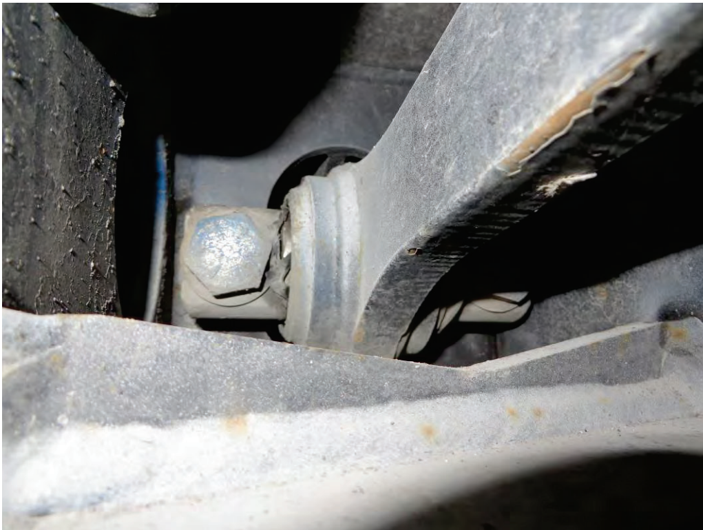
LOWER REAR TORQUE ARM BUSHINGS ARE WORN OUT (12,354 TEST MILES)
