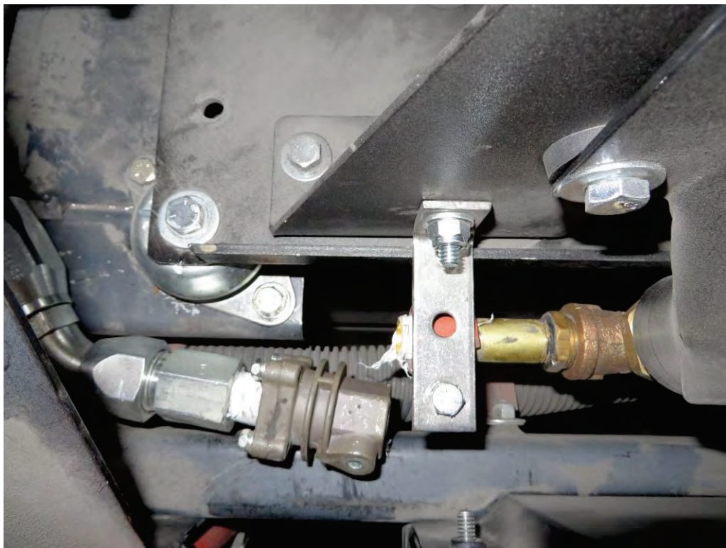
BRASS PIPE BROKEN ON SIDE OF AIR COMPRESSOR (12,443 TEST MILES)
