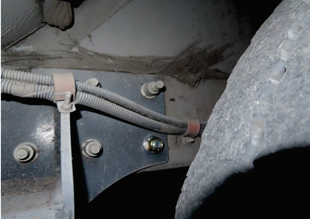
BROKEN HUCK BOLT REPLACED (11,491 TEST MILES)
