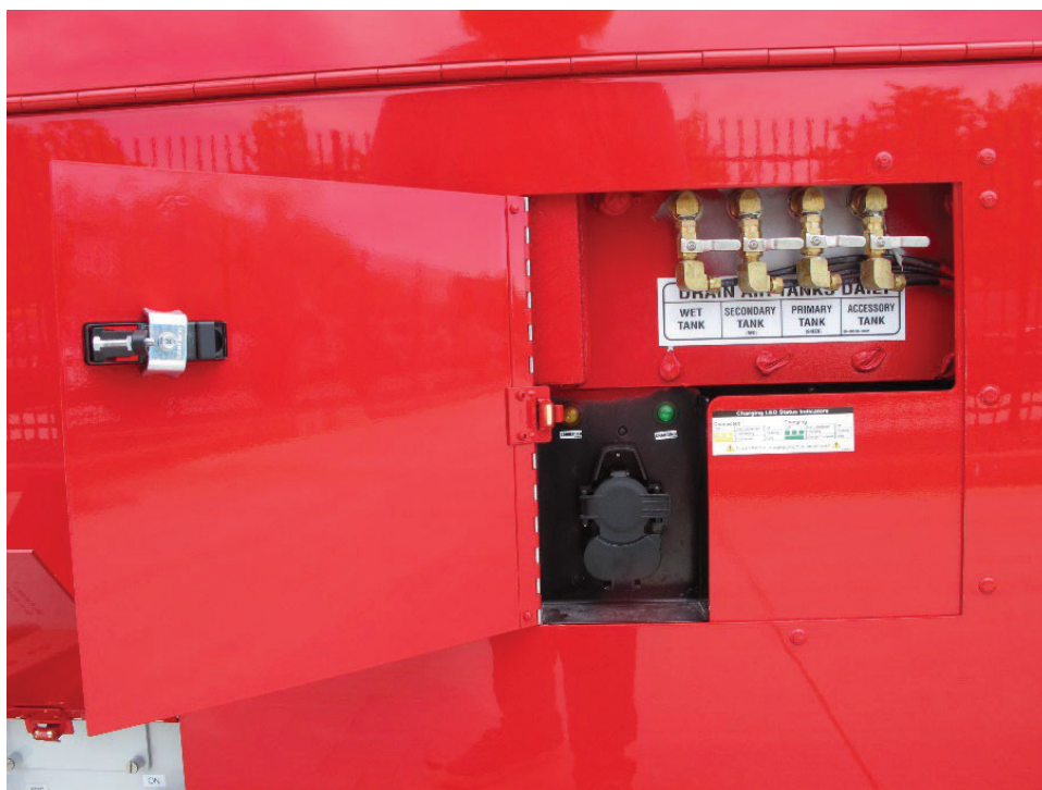
Streetside - Air Tank Drain Valves and Optional Plug-In Charger Location
