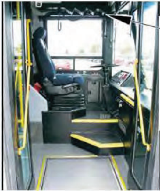
Drivers Area Highlighting Ergonomic Sawtooth Display Panel
