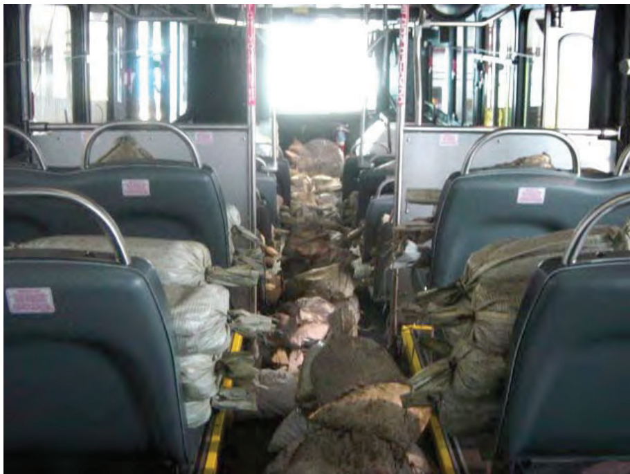
BUS LOADED TO 2.5 TIMES GVL (28,125 LBS)
