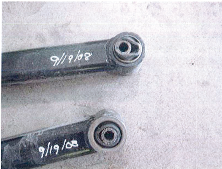
WORN BUSHINGS IN LOWER TRAILING ARMS (1,253 TEST MILES)
