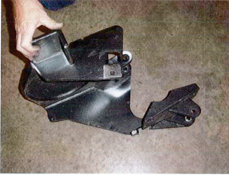
BROKEN RIGHT REAR AIR BAG PEDESTAL (2,661 TEST MILES)
