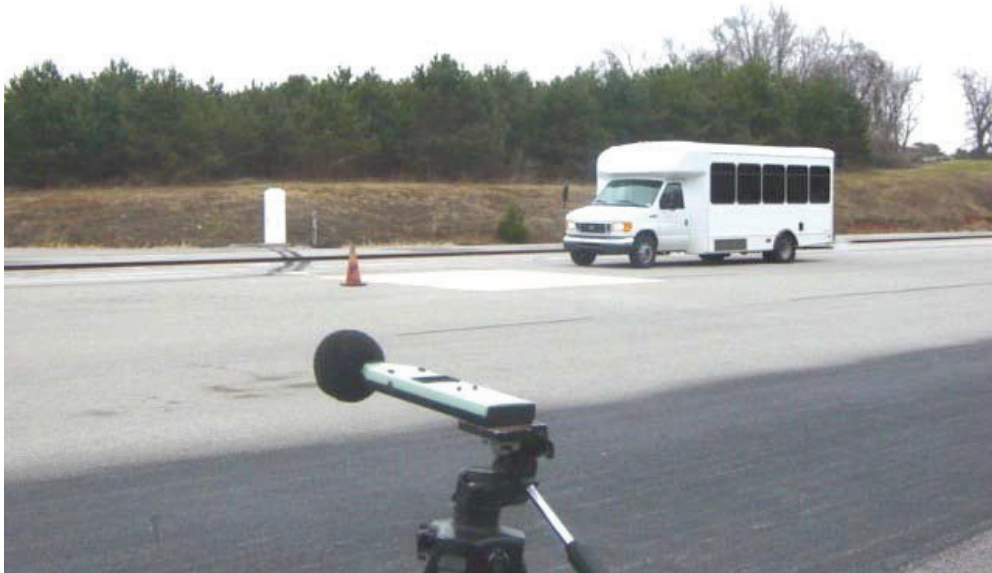
TEST BUS UNDERGOING EXTERIOR NOISE TESTING
