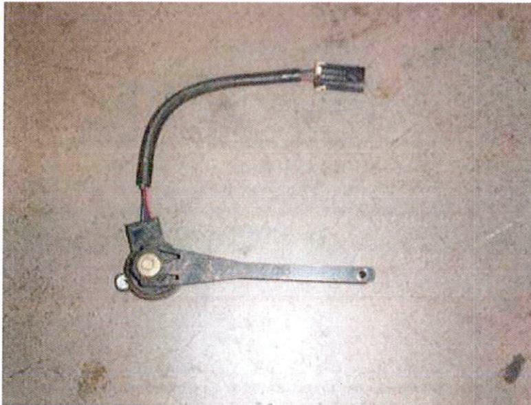
FAILED LEVELING VALVE (2,659 TEST MILES)
