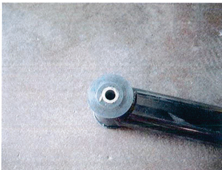
TRAILING ARMS INSTALLED WITH NEW TYPE BUSHING (1,253 TEST MILES)
