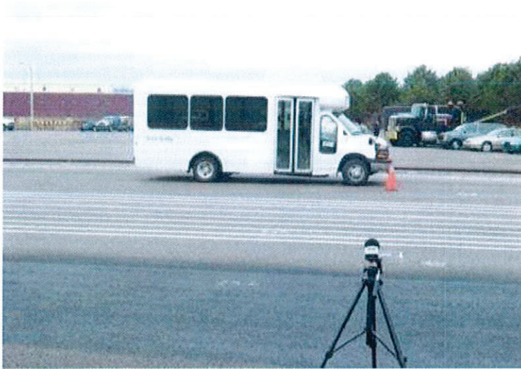
TEST BUS UNDERGOING EXTERIOR NOISE TESTS
