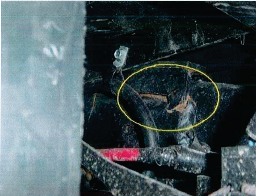
CRACKED FRAME RAIL (630 TEST MILES)
