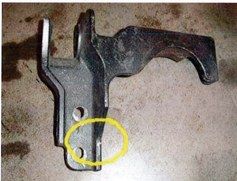
CRACKED REAR LATERAL BAR MOUNT (5,071 TEST MILES)
