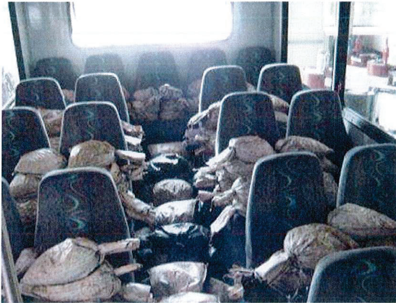
BUS LOADED TO 2.5 TIMES GVL (10,875 LBS)
